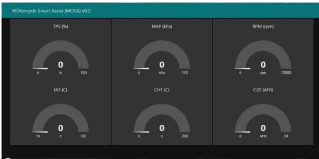
Figure 6. Snapshot of web-based UI produced by Dashboard UI node in Node-RED
