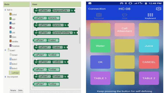
Figure 1. (a) Android App Setting (b) App layout An HC-08 Bluetooth module placed in the kitchen receives the order and display on LCD
