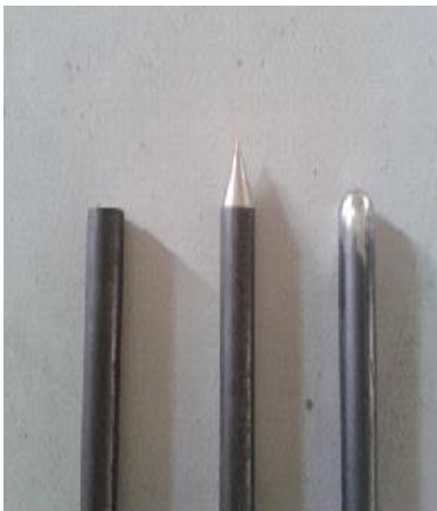
Figure 1. Different types of lightning rod, from left: flat, sharp and blunt surface
