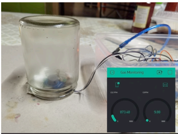
Figure 7. Functionality test on MQ-7
