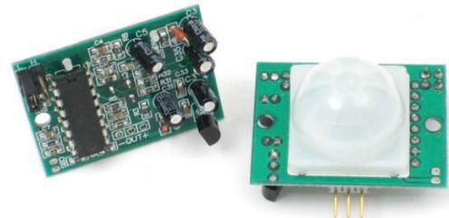
Figure 1. PIR motion sensor
