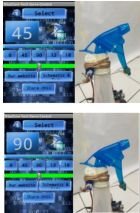
Figure 9: Servo Motor is Connected with 0° Initial States, 45°, And 90°
