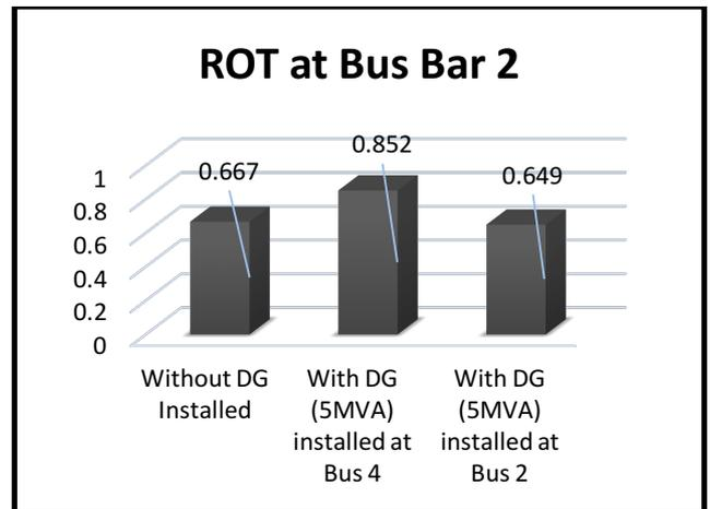
Figure 16. Comparisons of relay operating time at Bus 2 with and without installation DG of 5MVA
