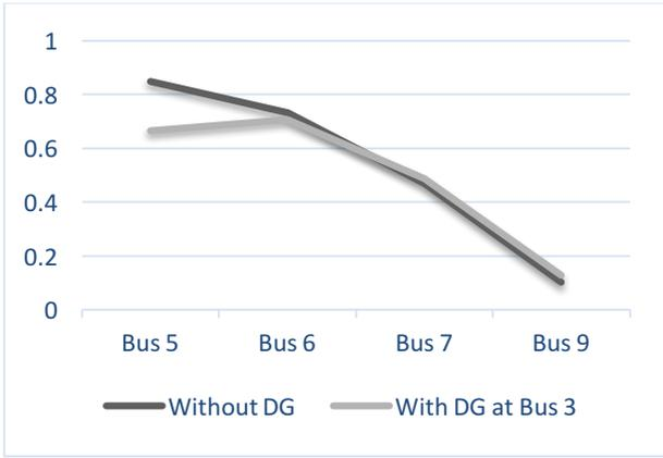
Figure 17. Relay Operating Time(s) versus busbar relay for case without DG and DG at Bus 3
