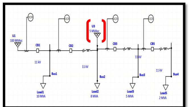
Figure 9. Circuit with Distributed Generation 5MVA Installation at Bus 2
