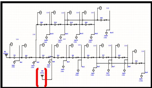
Figure 12: Circuit with Distributed Generation 8MVA Installation at Bus 3
