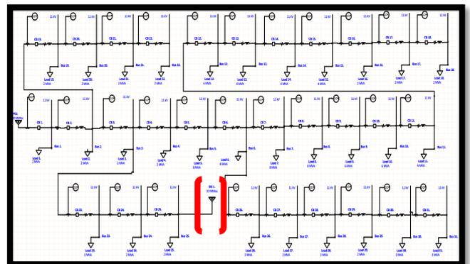
Figure 14. Circuit with Distributed Generation 10MVA Installation at Bus 25
