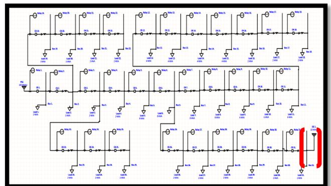
Figure 15: Circuit with Distributed Generation 10MVA Installation at Bus 31
