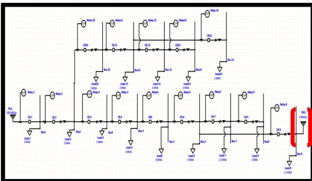
Figure 11: Circuit with Distributed Generation 5MVA Installation at Bus 8
