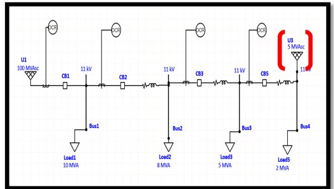
Figure 8. Circuit with Distributed Generation 5MVA Installation at Bus 4
