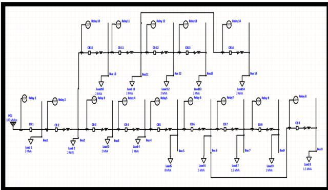
Figure 10. Circuit with no Distributed Generation Installation
