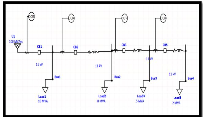
Figure 7: Circuit with no Distributed Generation Installation
