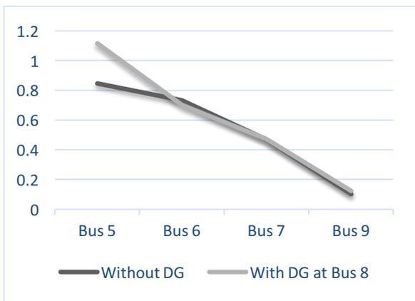
Figure 18: Relay Operating Time(s) versus busbar relay for case without DG and DG at Bus 8
