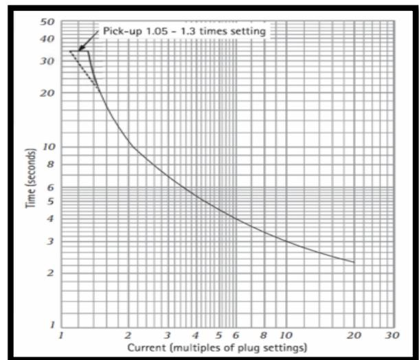
Figure 3. Standard IDMT Relay Characteristics
