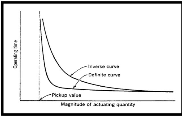
Figure 1. Relay Characteristic of IDMT Overcurrent Relay
