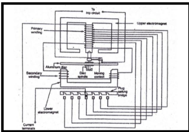
Figure 2. Structure of an Overcurrent Relay
