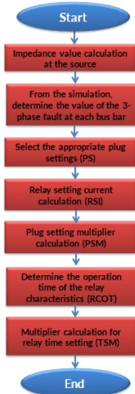
Figure 6. The IDMT Relay Settings are Determined Using a Flow Chart
