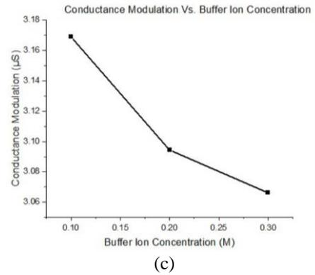
Figure 2. Conduction modulation against (a) radius (b) oxide thickness (c) buffer ion concentration of cylindrical nanowire biosensor
