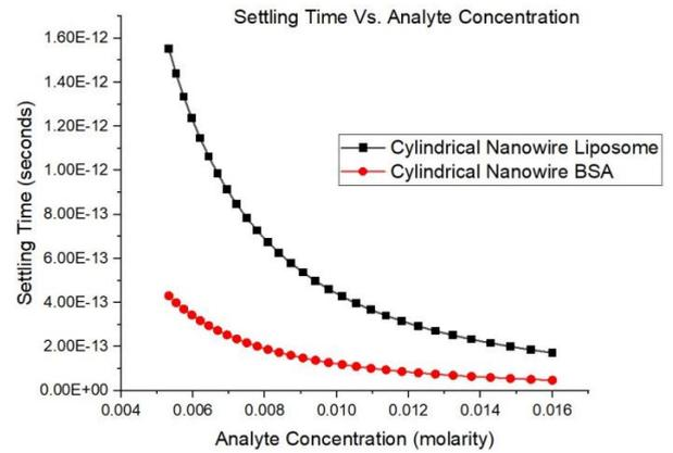
Figure 4. Settling time against Analyte Concentration of a cylindrical nanowire for liposome and BSA protein
