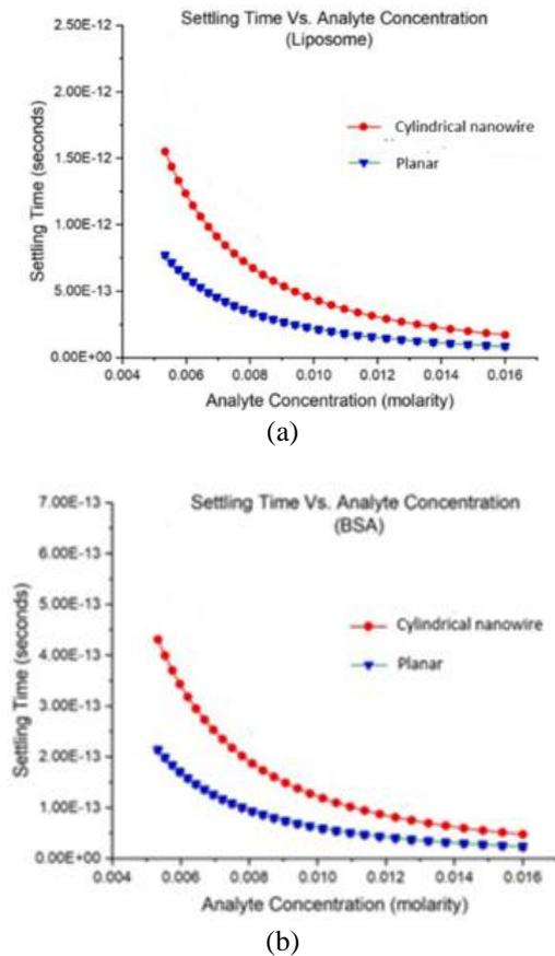
Figure 6. Settling Time against Analyte Concentration in Planar and Cylindrical Nanowire for (a) liposome (b) BSA
