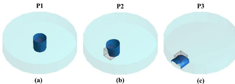
Figure 5. Synthesised isosurface representation of 3D reconstructed image of cube phantom at test positions P1, P2 and P3
