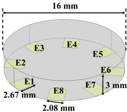
Figure 1. Sensor model of peripheral on-chip ECT sensor
