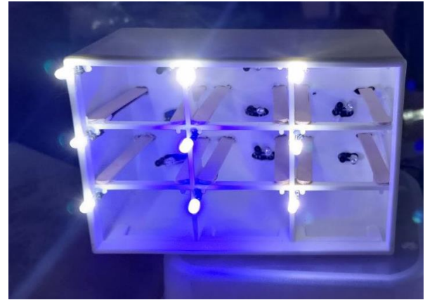
Figure 17. LED are lighting up when detecting pallet inside the compartment
