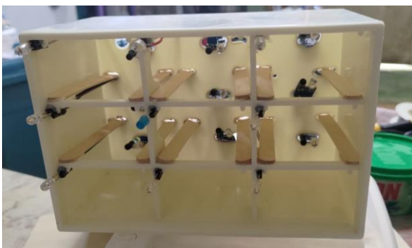
Figure 16. LED are not lighting up when no detection of pallet inside the compartment
