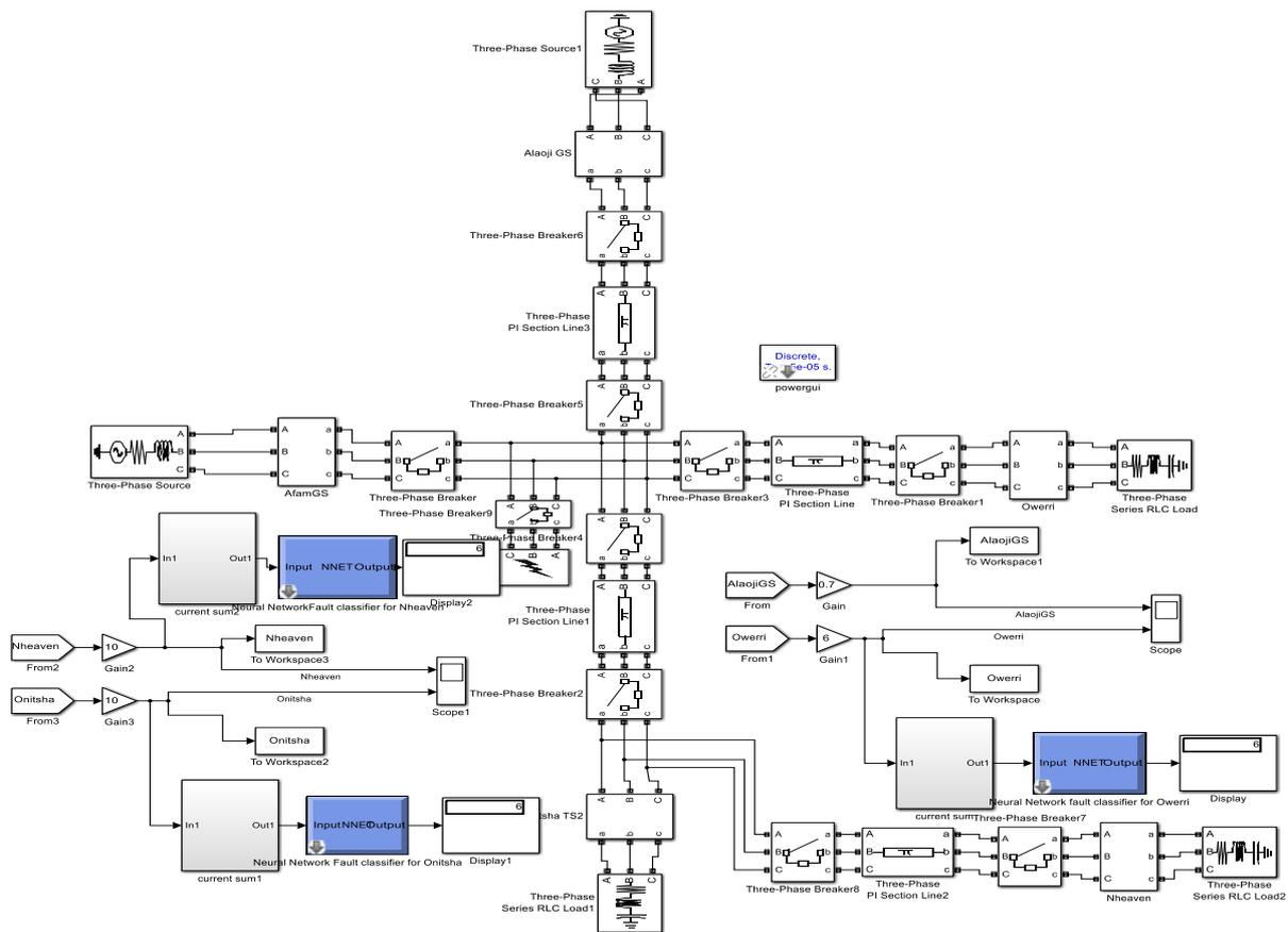
Figure 18. Power system model with ANN HIF detector and classifier with fault applied at the transmission line connecting Afam GS and Alaoji GS
