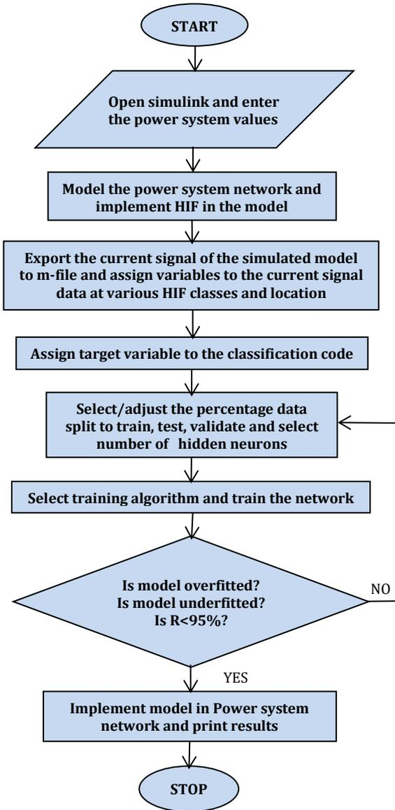
Figure 19. Flow chart of the modelling and simulation
