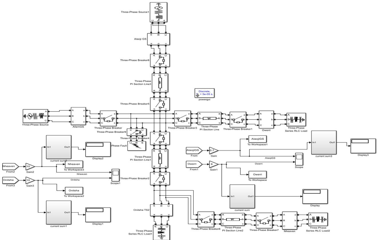
Figure 3. SIMULINK model of the power system Network with fault applied on the transmission line connecting Afam GS to Alaoji GS
