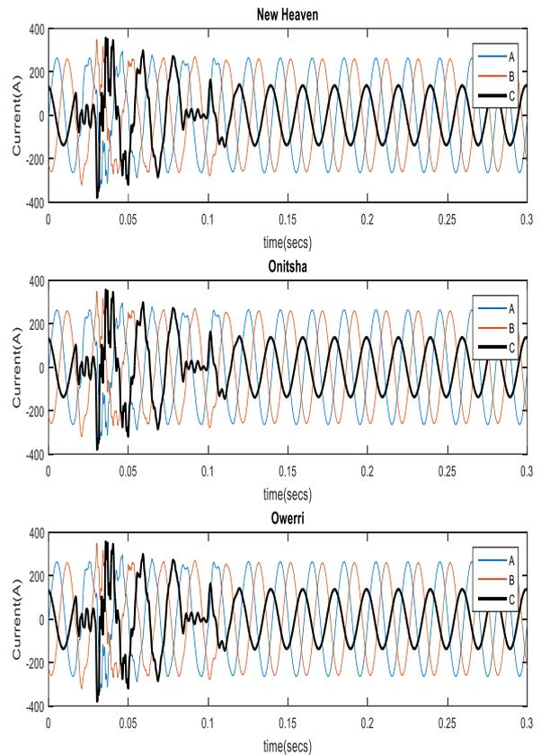
Figure 21. Current signal of HIF fault on a single phase
