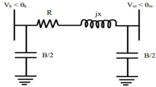
Figure 1. Transmission Line  $\pi$  circuit [17]
