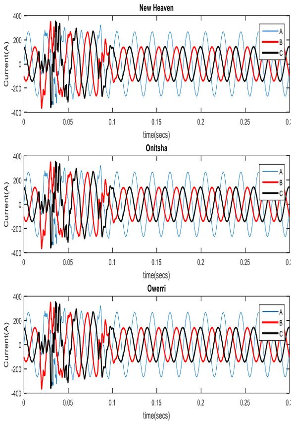
Figure 22. Two phase high impedance fault on the transmission line for each of the locations
