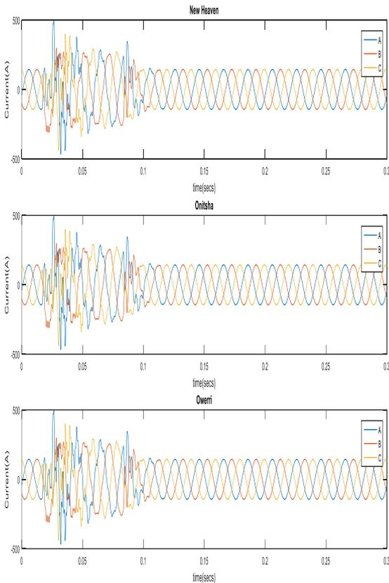
Figure 23. Three phase HIF on the transmission line network
