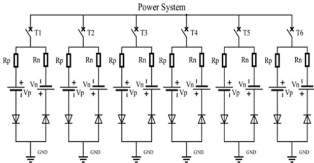
Figure 2. HIF model based on Emanuel arc model [18]
