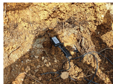
Figure 6. The installed soil moisture sensor
