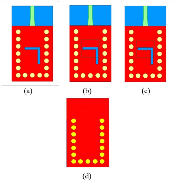
Figure 2. Antenna Design Evolution: Top view, (a) Stage 1, (b) Stage 2, (c) Stage 3, (d) Bottom
