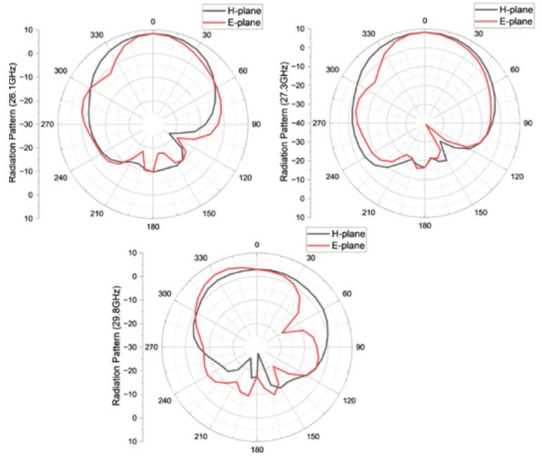
Figure 4. Radiation pattern E plane and H plane at resonant frequencies of 26.1, 27.3, and 29.8 GHz
