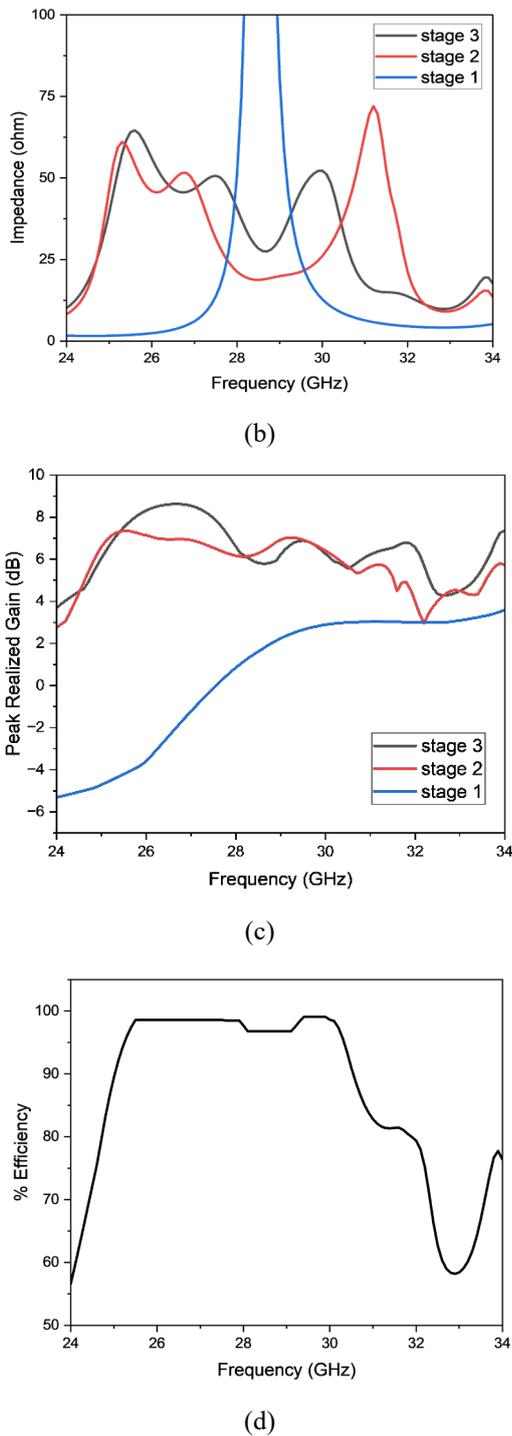
Figure 3. Simulated response for different geometry (a) Reflection coefficient, (b) Impedance plot, (c) Realized Gain, (d) Radiation efficiency
