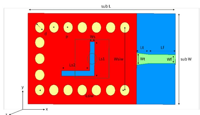
Figure 1. Single SIW DRA antenna with L-slot excitation
