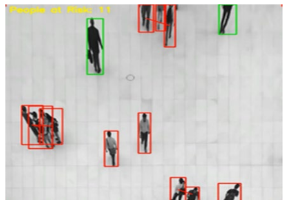
Figure 8. Output of physical distancing detection model using bird's view video frame
