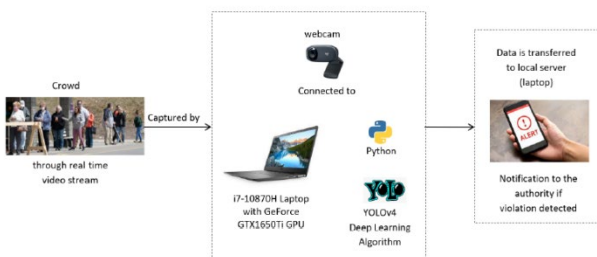
Figure 2. The block diagram of developing the physical distance and face mask-wearing surveillance system
