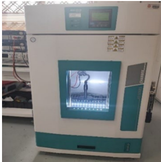
Figure 6. Top view of cylindrical cell inside thermal chamber
