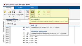
Figure 5. Convert the Simulation into a MATLAB App program
