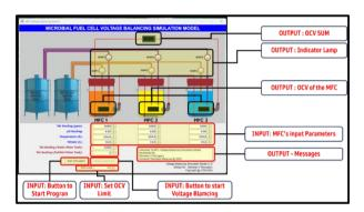
Figure 7. TCSSMFC Simulation Model Interface Screen
