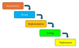
Figure 1. Modified Waterfall Model for Software Development
