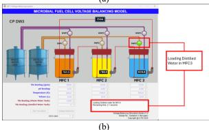
Figure 17. The result shows that the distilled water pump for (a) MFC2 and (b) MFC3 is turned ON
