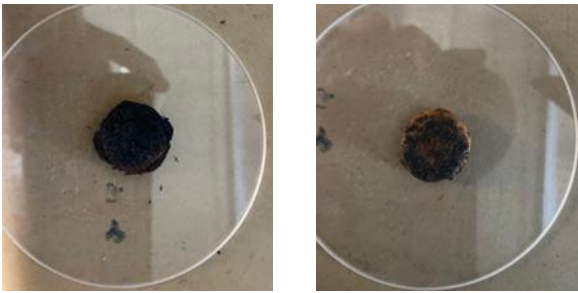
Figure 3. The condition of white bread when the applied voltage increases more than 13.6 kV.
