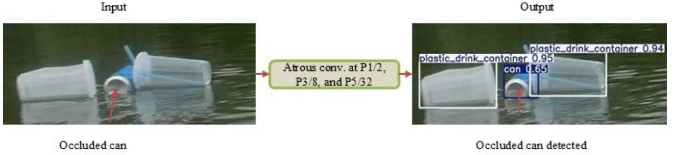
Figure 2. Effect of atrous convolution on detection
