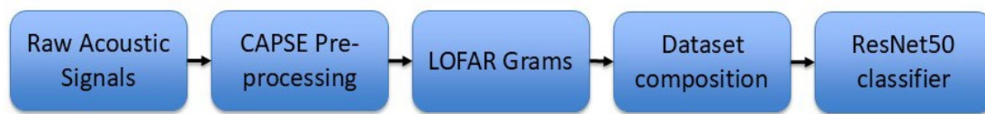
Figure 1. Overview of the classification pipeline showing acoustic input, preprocessing, and vessel classifier
