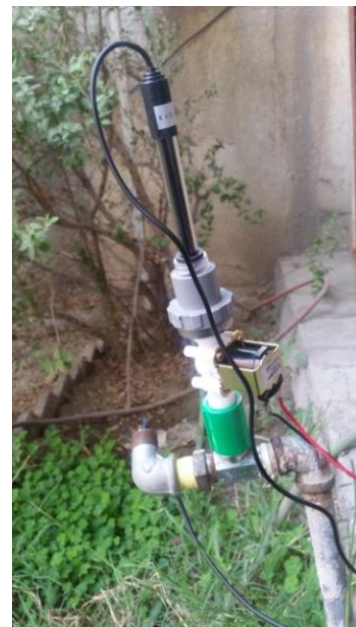
Figure 6. Solenoid valve associated with tap water in a home
